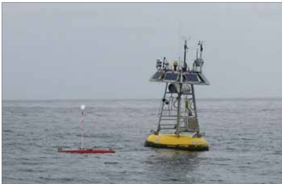
▲ Station keeping capability. An open ocean observation buoy ( right ) was moored next to a bottom pressure recorder (BPR) on the seafloor to relay data from the BPR to scientists on shore. Although it was moored beside the BPR, winds and currents tended to push the buoy to the southeast quadrant of its 3,400-m [11,000-ft] watch circle. A Wave Glider AMV ( left ) was tested for its feasibility as a relay station for the BPR data.
