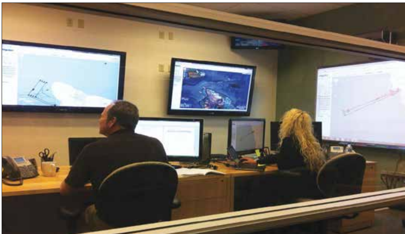
^ Pilot control station. At an onshore operations support center, pilots monitor vessel traffic, sea conditions and AMV operating parameters around the clock.
